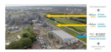
Advanced recycling at commercial scale at SABIC's world-first advanced recycling unit in Geleen, the Netherlands is now a significant step closer as our new hydrotreater plant has been successfully commissioned and has treated the first batch of pyrolysis oil, resulting in on-specifaction cracker feedstock which was then introduced into SABIC's OLE4 cracker. An evaluation will now be conducted to ensure the plant runs smoothly.
